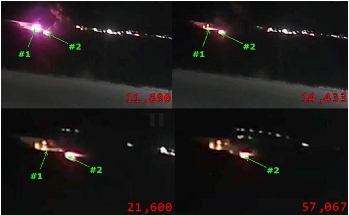
Figure 62. Fire plume moving into pool fire #2, as observed by the "Maliakos-Kleidi" camera.
