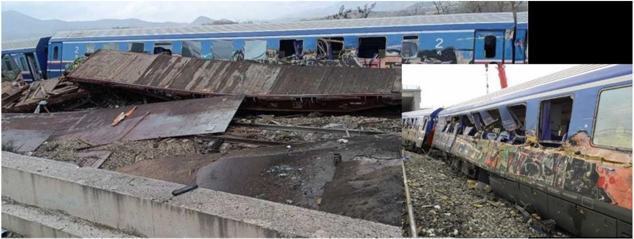
Figure 25. Linear impact of steel plates on the side of the coach B4.
